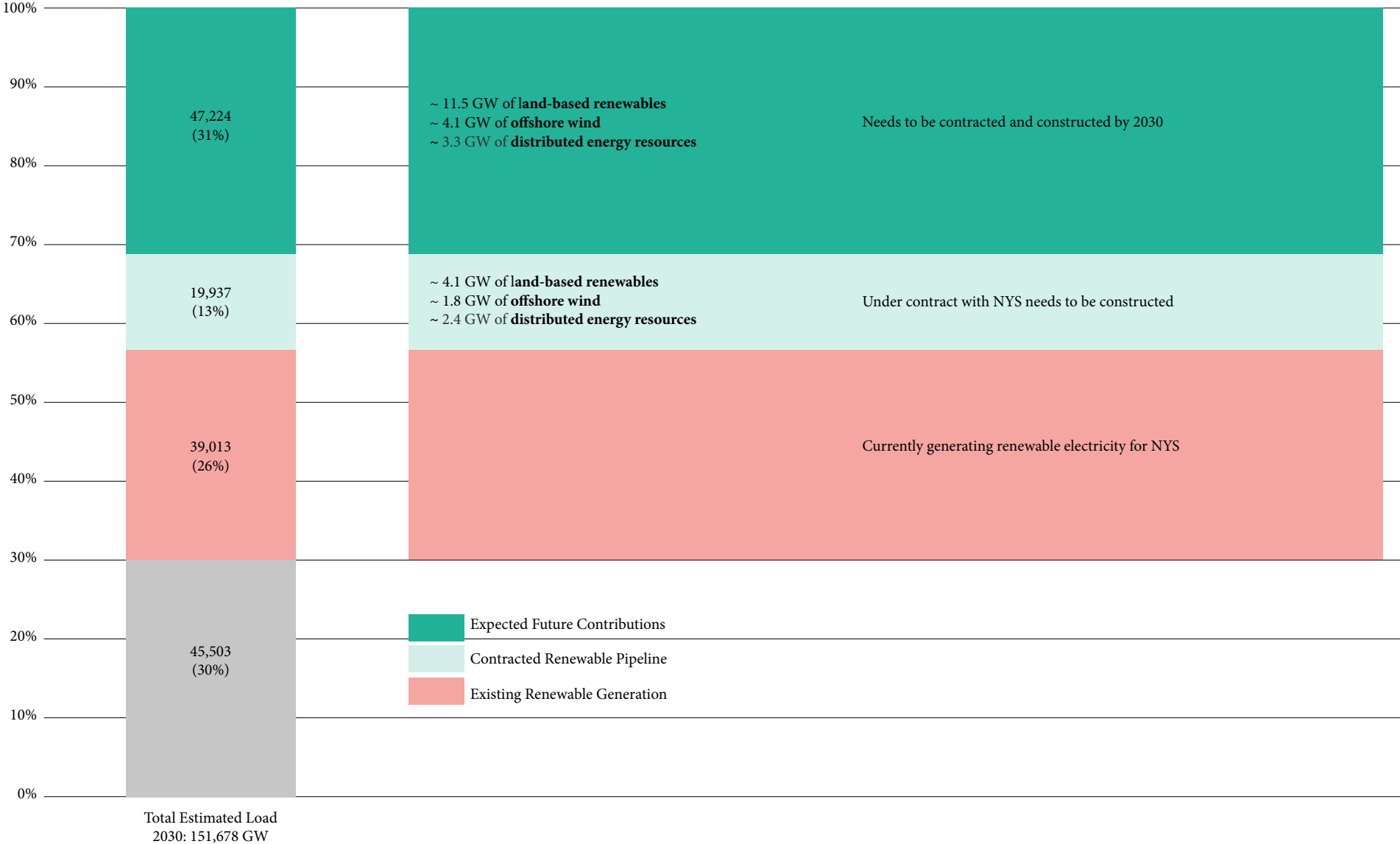
FIGURE 4. ESTIMATED RENEWABLE ENERGY DEPLOYMENT FROM 2020-2030 TO ACHIEVE 70% RENEWABLE ENERGY, graphic originally published from NYSERDA white paper, “Clean Energy Standard Procurements to implement New York’s Climate Leadership and Community Protection Act (July 2020).
